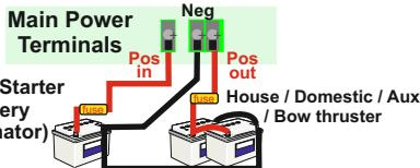
Ensure the charger is wired up as depicted above (larger diagram on previous page). The Pro Batt Ultra shall light up provided it has battery voltage across the **Pos in** and **Neg** terminal. If **Pos out** is also connected the unit shall start charging for 120 seconds (1/2 of the regen. braking timer). During the first start up you can change the battery chemistry profile.
