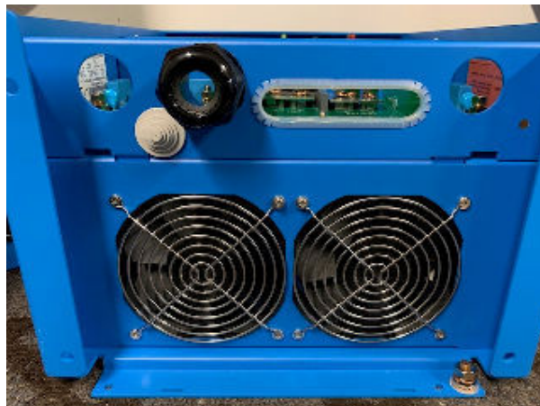
Figure 7 - 5kVA Blue Fan Cover Plate Removed
