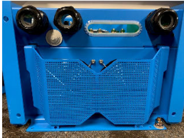
Figure 6 - 5kVA Blue Fan Cover Plate Installed
