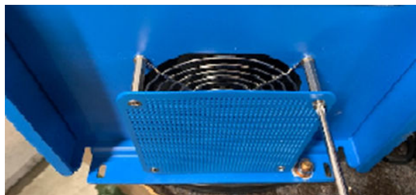
Figure 4 - 3kVA Blue Fan Cover Plate Installed
