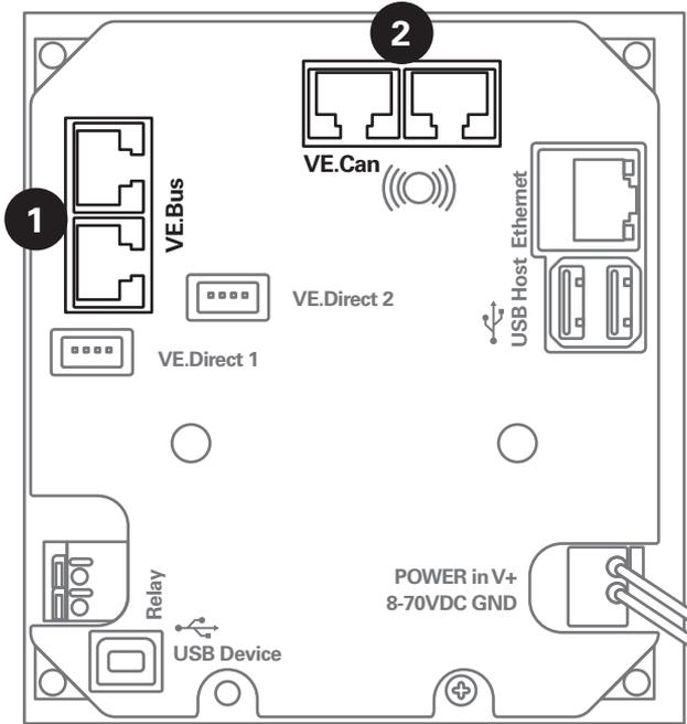
**Figure 5. Victron GX device**
