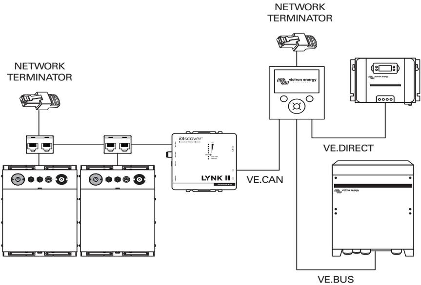
**Figure 1. Example LYNK II with Victron Energy devices**
