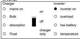
The inverter is on, and supplies power to the load.
