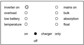
**Note:** When the LED's "overload" and "low battery" are on simultaneously, the Multi(Plus) or Inverter Compact has switched off due to excessive DC ripple voltage.
