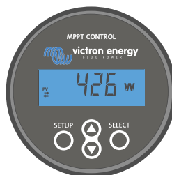
The MPPT Control display
