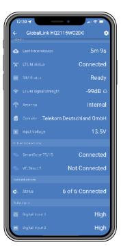
On the status screen there is information about the connectivity to the LTE-M network and the Victron Remote Management portal. For the device to work properly, the SIM status should be Ready and the LTE-M status must be Connected. You can also check if the correct antenna is selected and the current signal strength. The status screen also shows the operator name and number. It is not possible to select one yourself, even if more than one network is available in your region.
