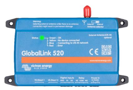
The GlobalLink 520 allows you to connect other Victron equipment, such as your Battery Monitor (BMV), SmartShunt, Solar Charger, Phoenix Smart IP43 Charger or Phoenix Inverter to the Victron Remote Management (VRM) portal via VE.Direct or Bluetooth. RuuviTag and RuuviTag Pro sensors via Bluetooth Low Energy (BLE) are also supported. The VRM portal is available to use free of charge to view the status of your installation from anywhere in the world using your desktop or mobile device.
